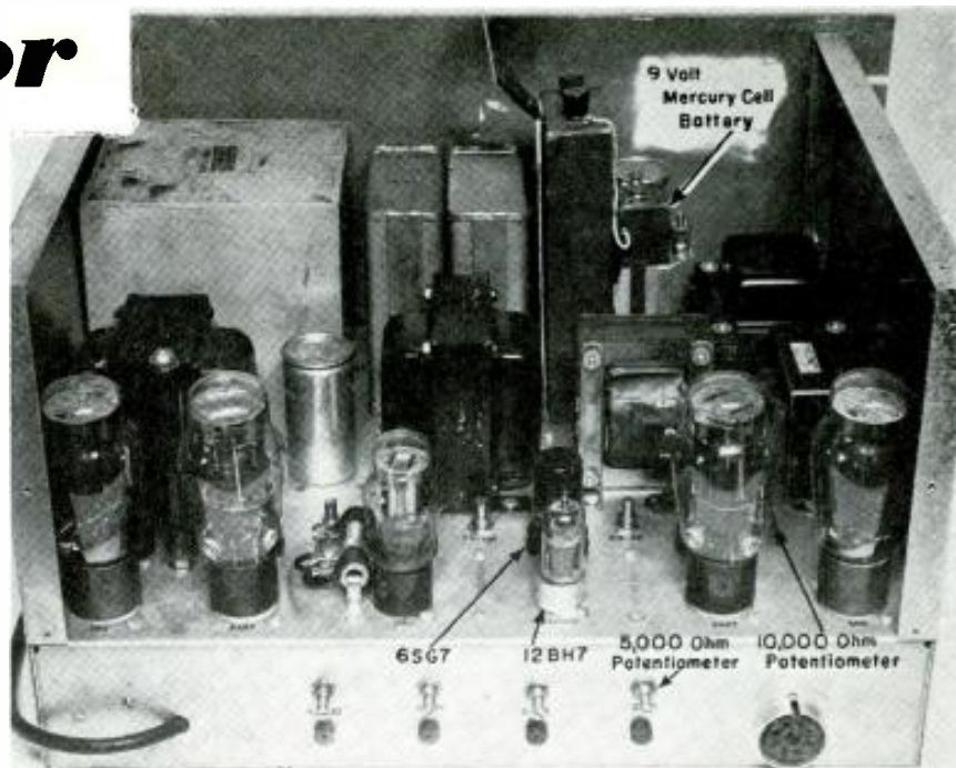
Figure 3 MULTIVOLTAGE SUPPLY incorporating the 12.5-volt regulator. The pin jack directly beneath the 5000-ohm potentiometer on the rear of the chassis is used for monitoring output voltage when adjusting the regulator.
