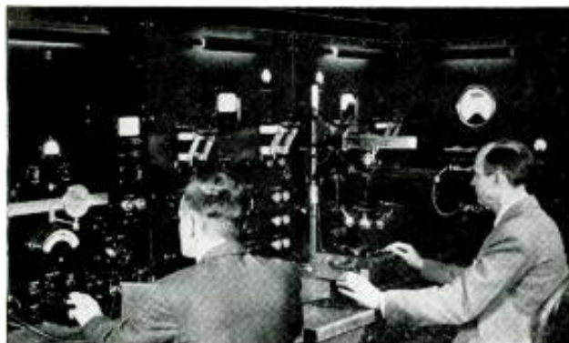
AUDIO FREQUENCY measurement standards, developed at Bureau of Standards, featuring a highly accurate electro-thermic transfer standard for the measurement of voltage and current.
